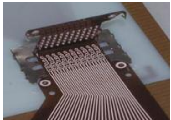
High density flexible substrate connection using a UTF Connector concept model
